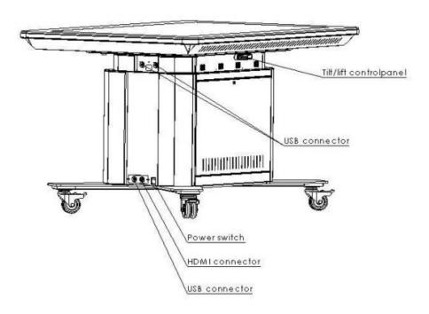
The Sectra Table has several connections and buttons. On the outside of the Sectra Table, the following can be found:
